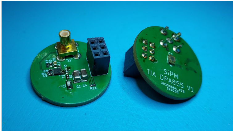
Figure 7: Assembled detector module. PCB is designed to fit in a 1 inch lens tube for ease of alignment.
