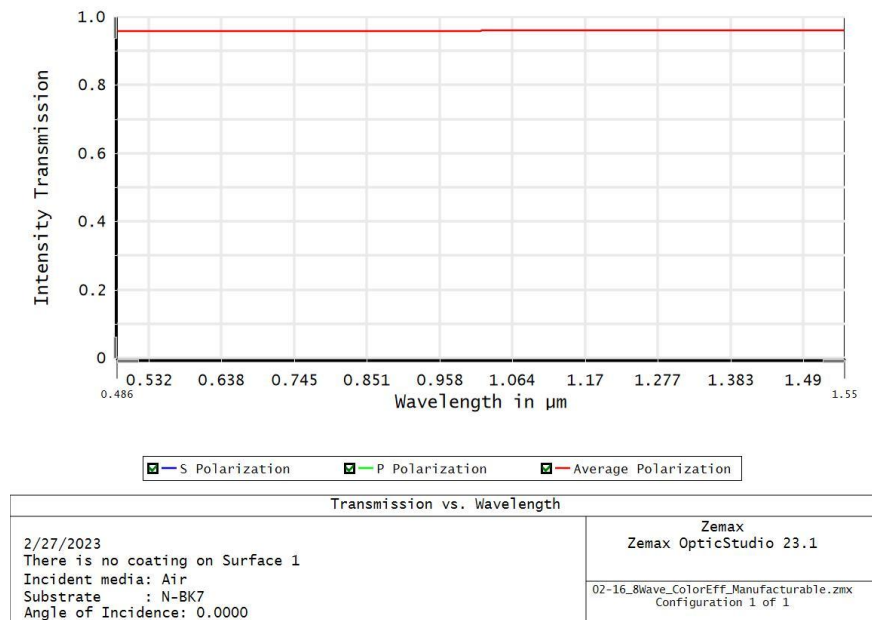
Figure 11.1: Intensity transmission plot of a single N-BK7 surface vs wavelength
