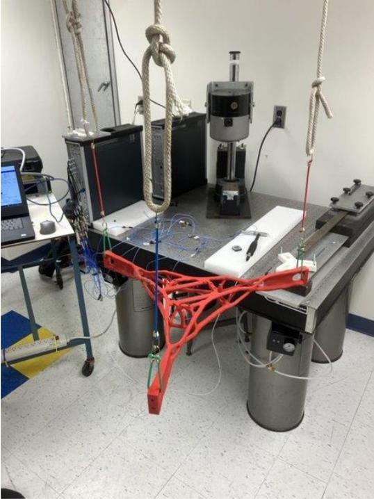
Figure 10: Strike modal test experimental set up. Concept A is hung off the ground with bungee cords for free-free constraints.
