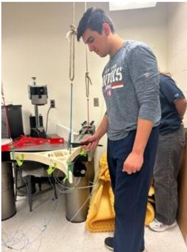
Figure 67: Hammer test set up.
