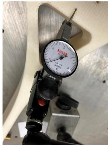
Figure 65: Set up and measurement for deflection test with 8.9 lbf load.
