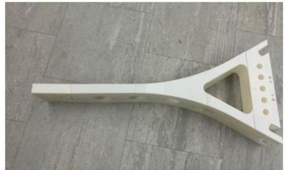
Figure 63: 3D printed arm with 3-inch of lattice infill. The arm was printed in sections that fit together.
