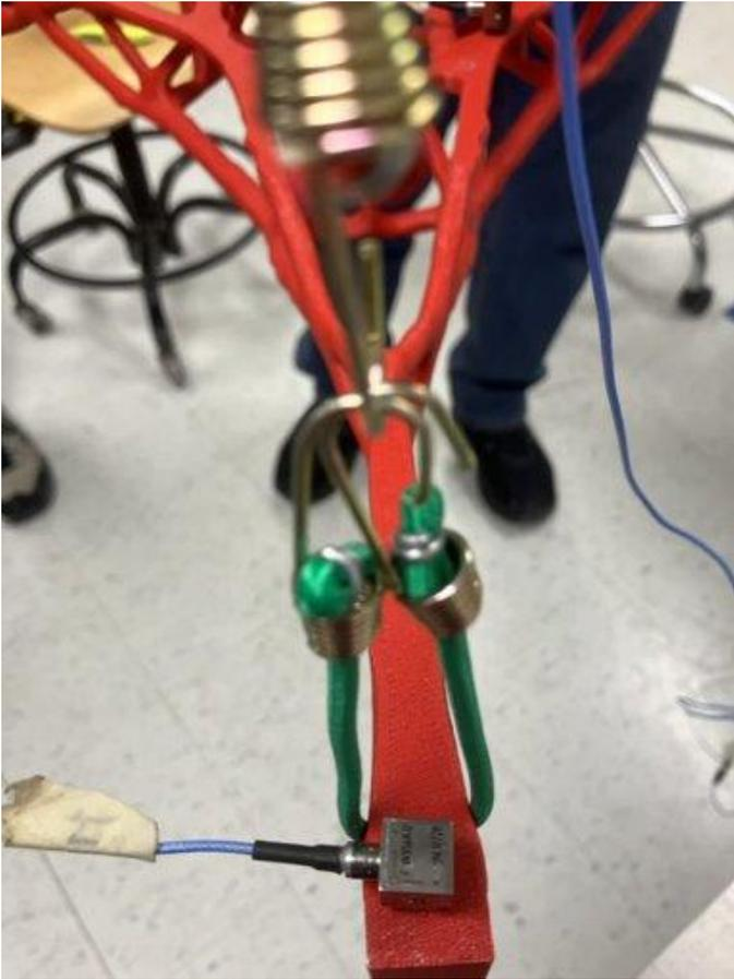
Figure 11: Accelerometers placed on Concept A for strike test to record data.
