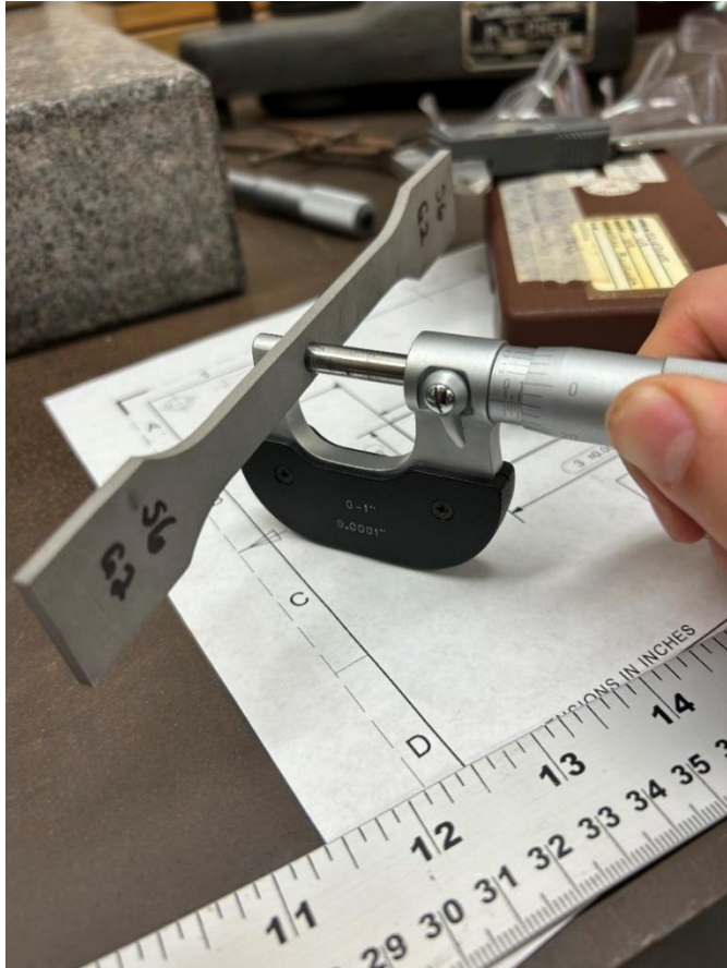
Figure 26. 3D Printed Coupon Gage Thickness Measurement with Micrometer on a Steel Coupon.
