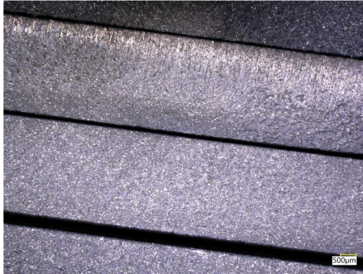
Figure 24. Group 4 Steel Coupons (4 total in Group). The Sandblasted Finish can be Faintly Seen on the Second Coupon From the Top.
