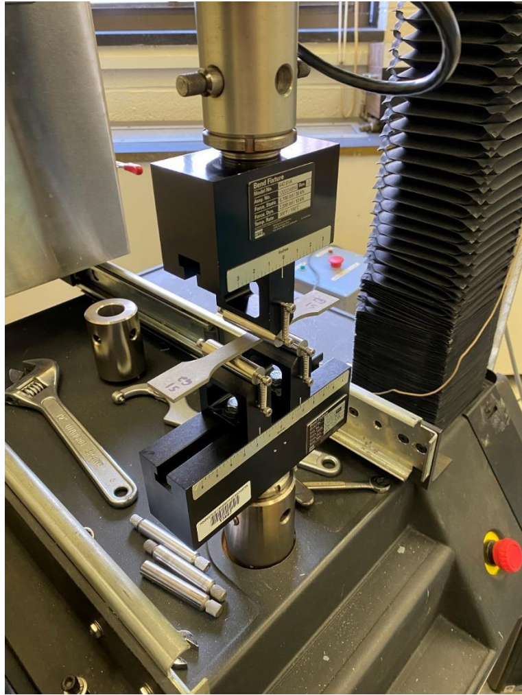
Figure 31. The 3-point Bend Test Setup on the MTS Machine With a 3D Printed Steel Coupon.
