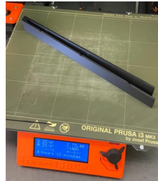
Figure 5. Sections of 55% Scaled Model of Concept 3 to Test In-House Printing.
