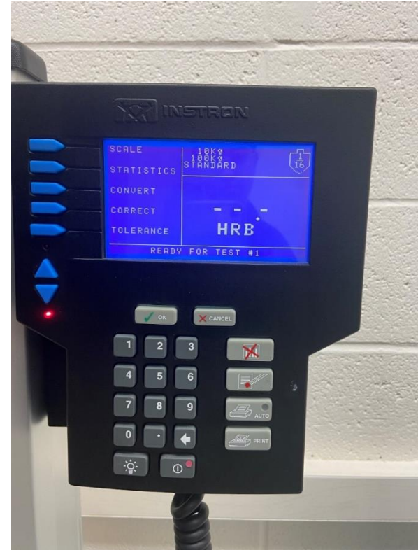
Figure 30. Rockwell Hardness Test Screen Setup for the Scale B 1/16-Inch Steel Ball Indenter With an Applied Force of 100 kg.
