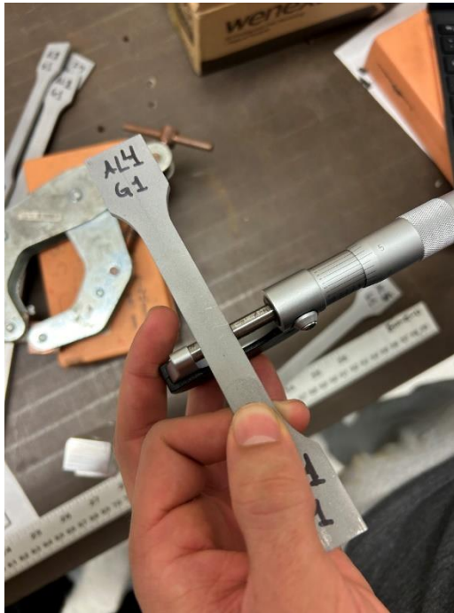
Figure 25. 3D Printed Coupon Gage Width Measurement with Micrometer on an Aluminum Coupon.
