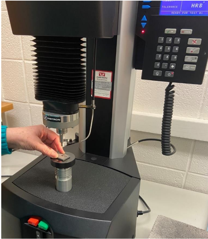
Figure 29. Rockwell Hardness Test Setup With one of the 3D Printed Steel Coupons.
