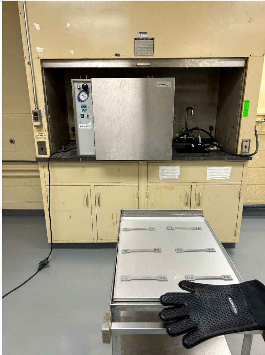
Figure 28. Thermal Cycling Setup. The Group 2 Steel Coupons are Pictured Prior to the Start of the First Thermal Cycle.
