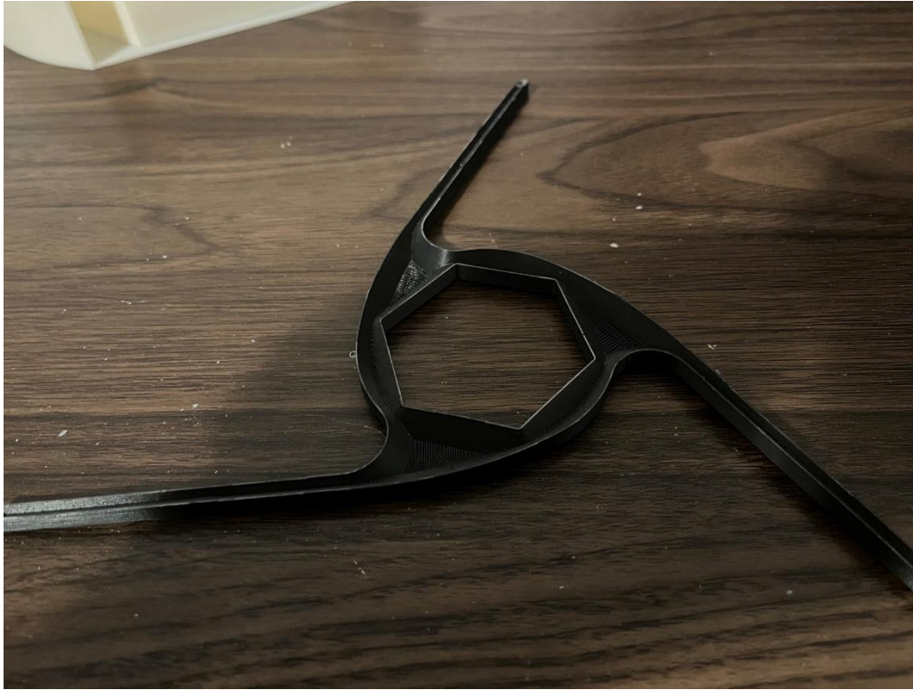
Figure 7. Print of 10% Scale Model for Proof of Overhang Angle Concept in Full Model.
