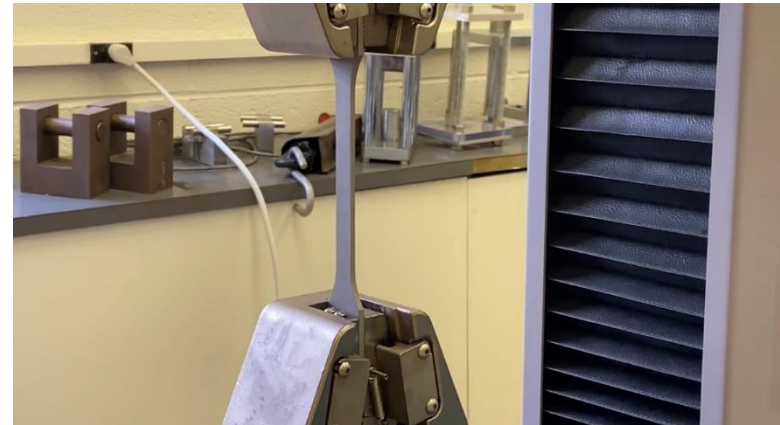
Figure 32. Tensile Test Setup on the MTS Machine With a 3D printed Steel Coupon in the Grippers.
