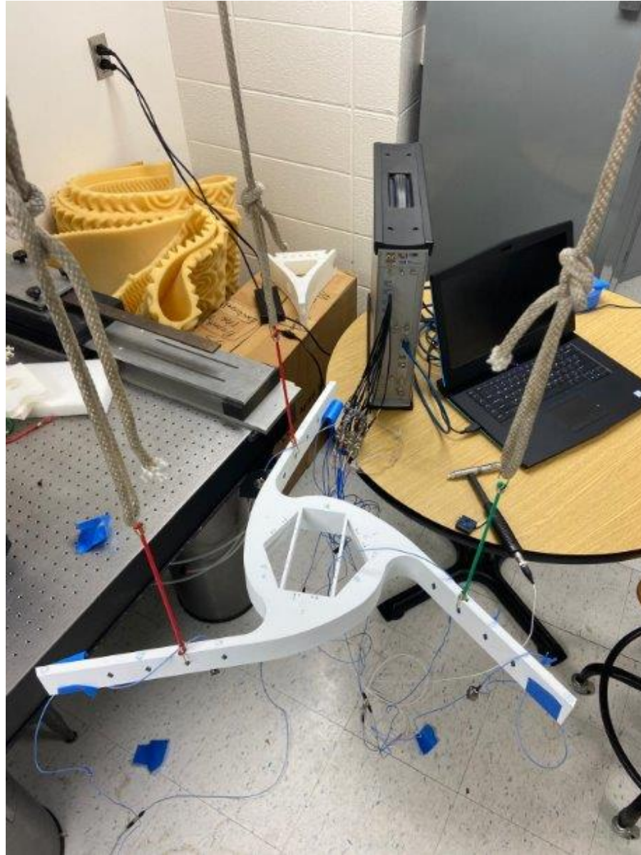
Figure 47. The Modal Strike Test With the Hanging Setup.
