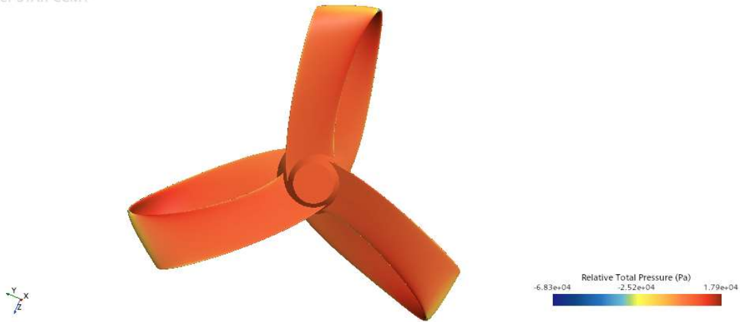
Fig. 26: Relative total pressure plot for the final toroidal model running at 5.5 rev/s (300RPM).
