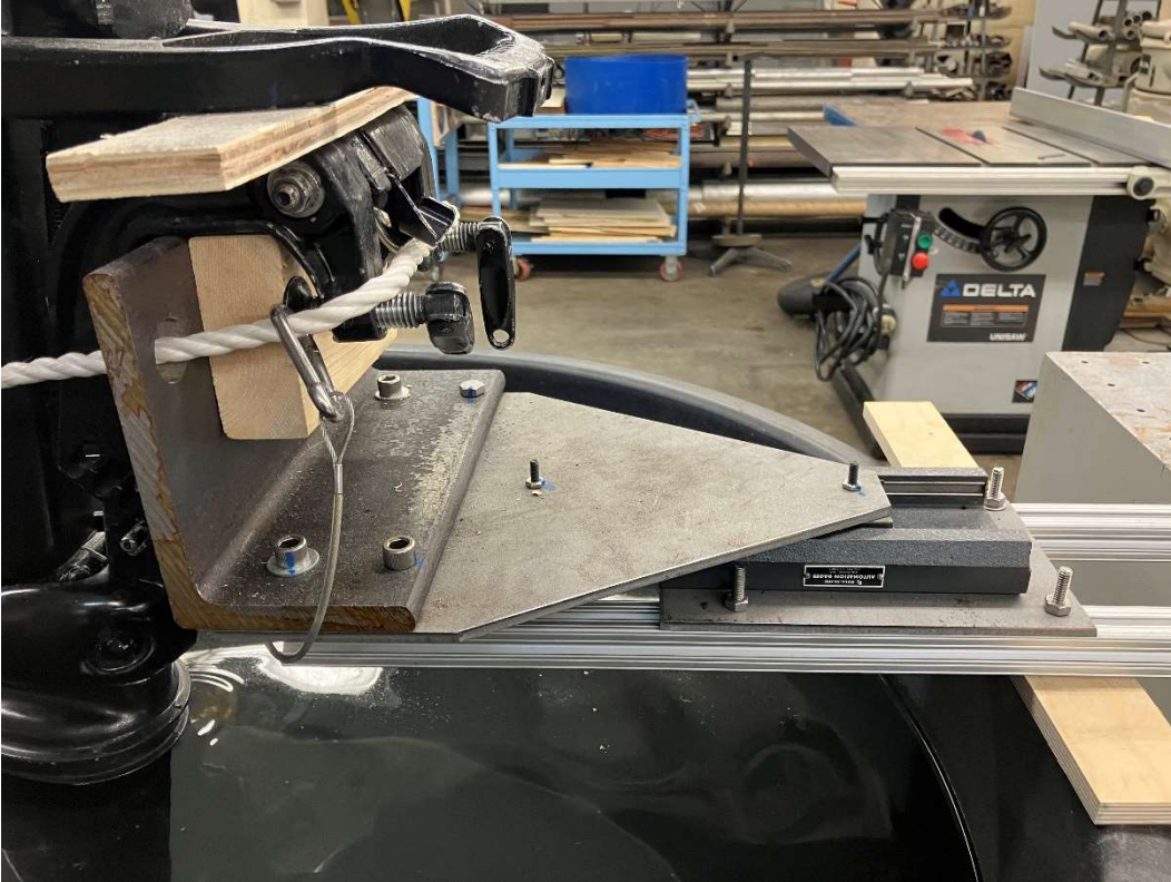
Fig. 5: The motor mount and uniaxial slider in the testing rig.
