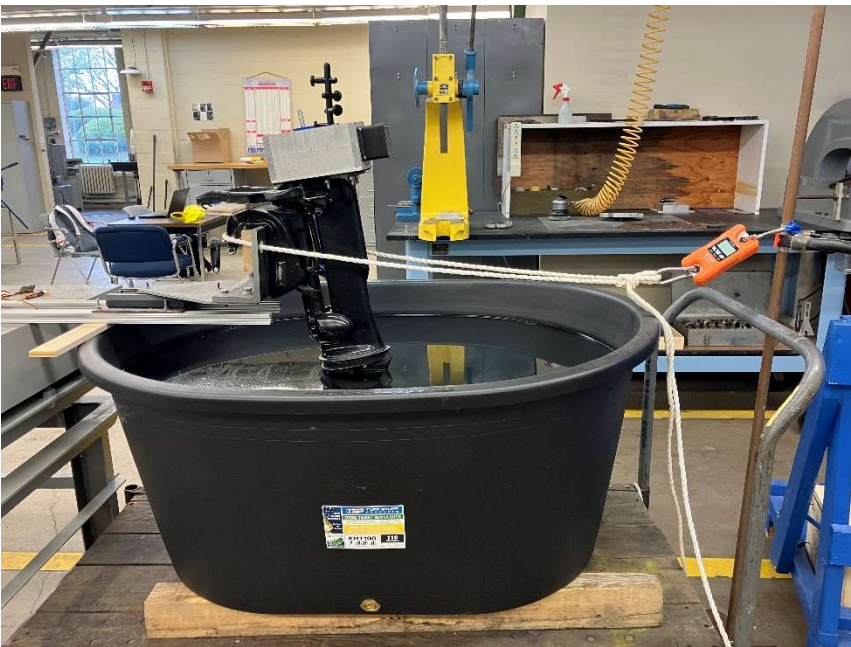
Fig. 6: The assembled testing rig setup.
