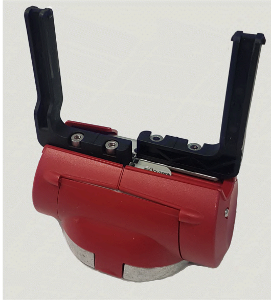
Fig 3. Current parallel jaw end effector used on Baxter & Sawyer robots [1]
