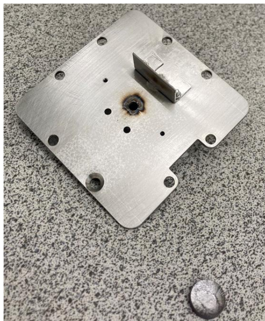
Figure 11. Image of front plate after the first laser shot. The mirror is coated with aluminum that was blasted through the light relay.
