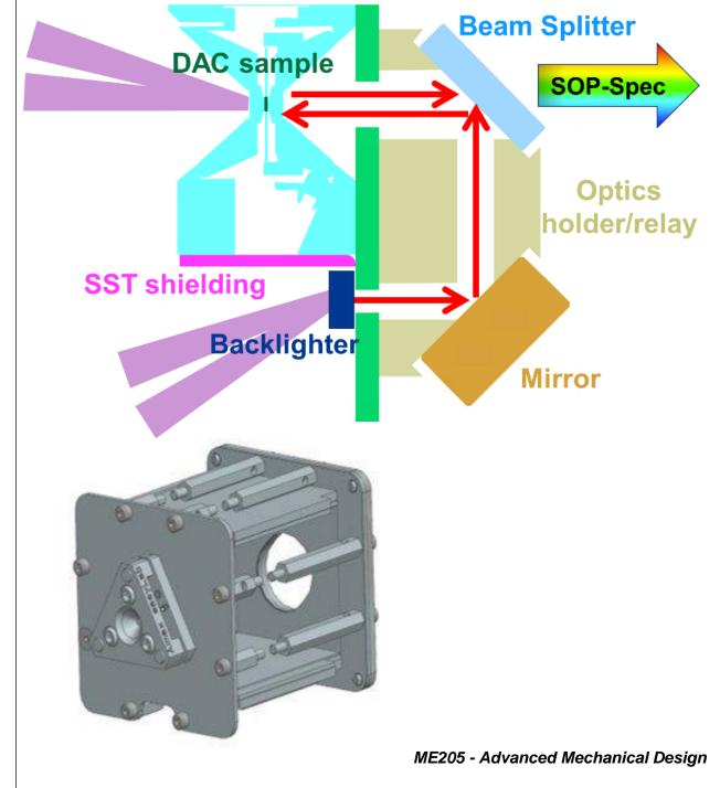
As the core component of the design, the reflectivity box used to relay the light had various concepts developed, varying primarily in their geometry.
