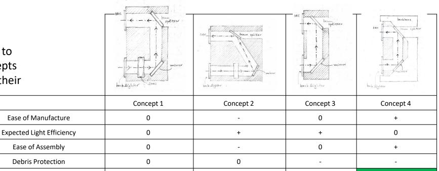
Concept 4 was selected, which utilized a backbone to hold the reflectivity box (in red) to the front plate.
