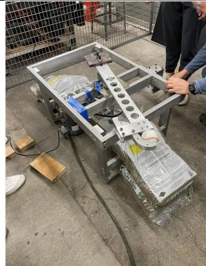
3. The next step is to attach the bat to the setup. This is done by lining the knob of the bat with the head of the shoulder bolt. The U-Bolt should then be tightened to secure the bat to the holder.
