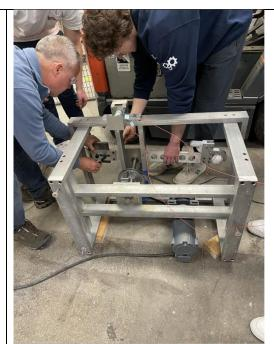
2. The next step is to secure the ball into the release mechanism. This is done by latching the release mechanism and then pushing the ball into place. The distance between the top of the baseball and the top of the release mechanism should be held constant for more accurate testing.
