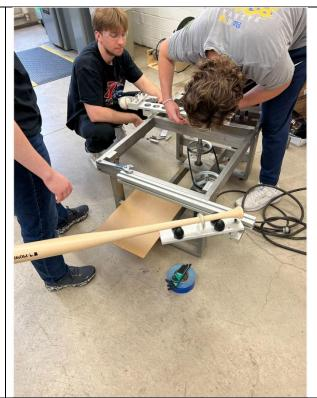
4. After the bat is in place, the high-speed camera is placed into position. The camera requires lots of light to clearly see the collision. The position of the camera can be tested by holding a ball to the spot of collision on the bat and adjusting the camera to see the point of contact.
