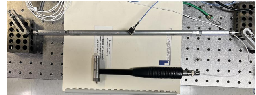
Hammer test for frequency response on Struts Assembly
