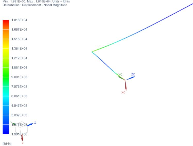
Figure 6, Strain energy plot of mode 3
