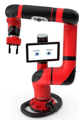
Figure 2. Sawyer Robot with existing parallel gripper
