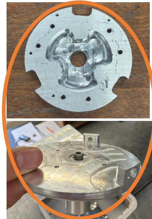
Figure 17. More material can be removed to save weight, and method of hole alignment could be improved.
