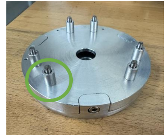
Figure 18. The two base plates joined with the risers.
