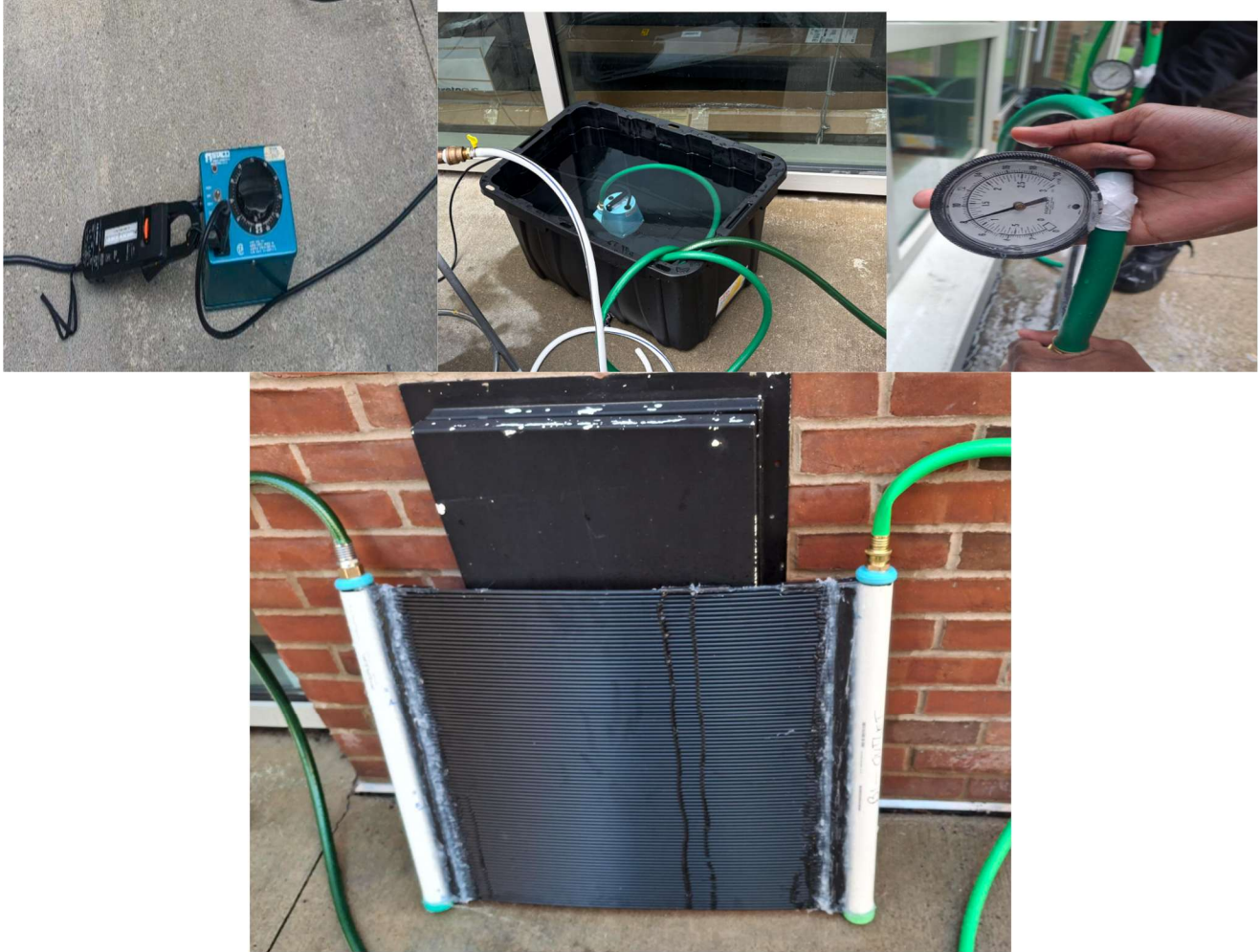
Figure D6: Experimental test rig components. Top (left to right): Variac and ammeter for pump voltage regulation, water reservoir containing the submersible sump pump, and analog pressure gauge for inlet monitoring. Bottom: Assembled 50% scale manifold and panel model during flow testing.
