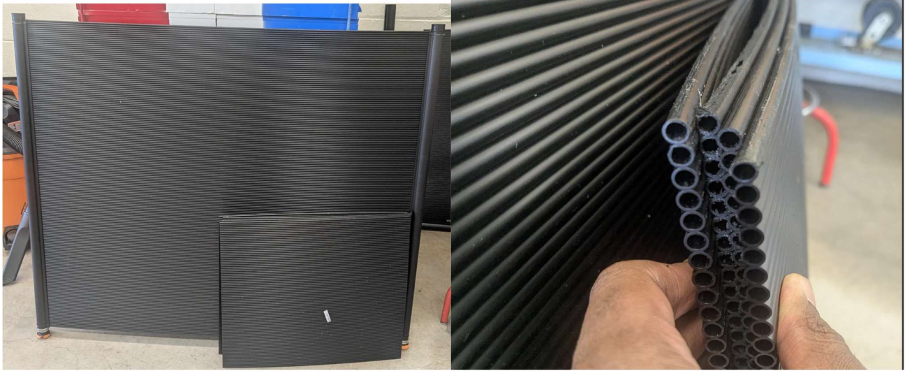
Figure D5: Comparison of the full-scale MicroEra heat exchanger panel and the 50% scaled test models. The smaller manifolds shown in the foreground were utilized for physical flow testing and volume collection experiments to validate the "choking" strategy developed in MATLAB and CFD simulations.
