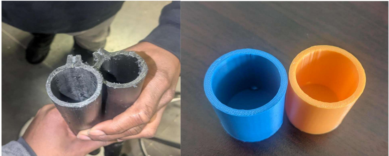
Figure D2: Comparison of prototype manifolds used in discharge testing. The left images show the initial black manifolds where insufficient cleaning/deburring led to a negligible 1.8% flow improvement. The right images show the 3D-printed scaled models (blue and orange) with precise re-entrant orifices. These clean models demonstrated that under higher internal pressure at lower depths, discharge velocity improved by 26%.
