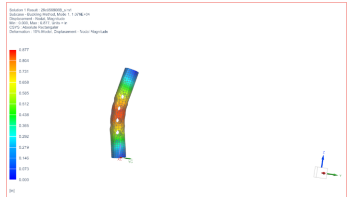
Figure 15: FEA Simulation of shorter struts. Stress-Element-Nodal results of manufactured strut. Solution 105, CQUAD4 (.0833 in mesh), Al 6061 (NX Library). FOS determined to be 1.076E4 psi under 1 lbf axially. Same boundary conditions and constraints present as Figure 14.
