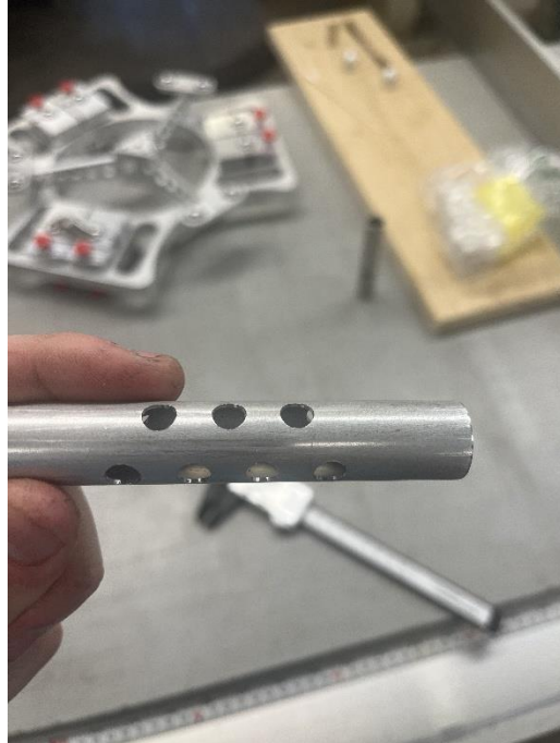
Figure 30: Close up view of the strut connecting the PMM and camera mount. Final lightweight design.
