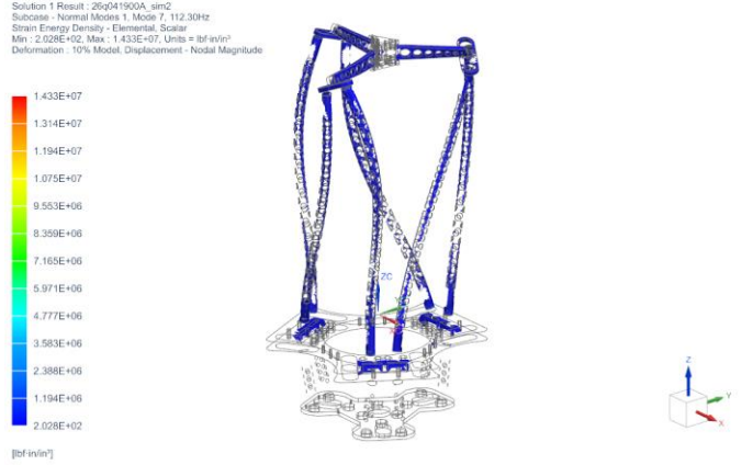
Figure 23: Strain energy density of the assembly from the first mode. SOL 103, Al 6061, CTETRA(10), mesh sizes of .3" and .7" present.
