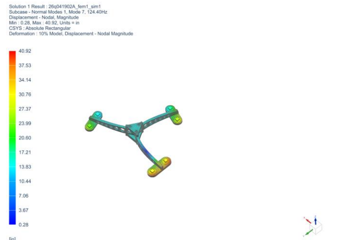
Figure 19: SOL 103 Real eigenvalue analysis, displacement results for the secondary mirror mount utilizing CQUAD10 elements. Al-6061 used as material
