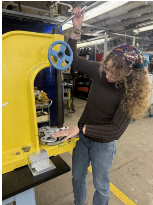
Figure 31: Press fit process of steel balls into camera mount
