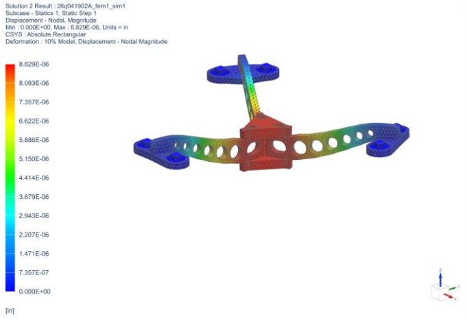
Figure 20: SOL 101 statics NX displacement results, for objects meshed using CQUAD 10 elements. Al-6061 used as the material.
