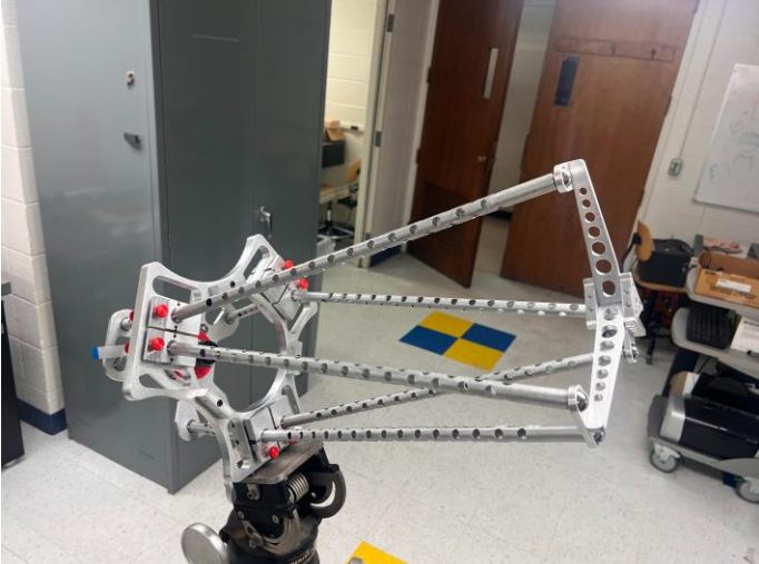
Figure 32: Final assembly on satellite mount. Matches fixed constraint present in assembly simulation. Light weighted struts can be seen in the center of the frame along with the PMM and SMM.
