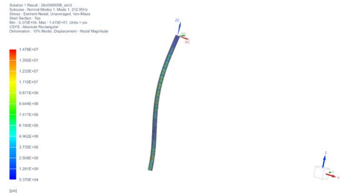
Figure 14: Modal results (Solution 103) of the longer struts. RBE2's were used at either edge simulating the ball joint. SPC12 is present at the top and SPC1236 is at the bottom. CQUAD4, .1" mesh size, Al-6061 (NX Library). First mode of 212.95 Hz
