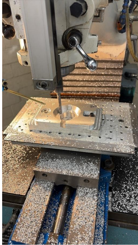
Figure E5: Bottom conical fixture being made on ProtoTRAK mill.
