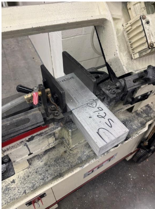
Figure E2: Stock piece being cut by horizontal bandsaw.
