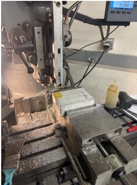
Figure E1: Riser cone being faced off on manual mill.
