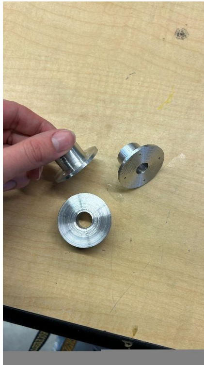
Figure E4: Custom couplers that transfer rotational motion from a servo motor to a lead screw.
