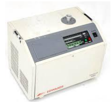
Edwards Spectron 600D leak rate tester can verify vacuum sealing
