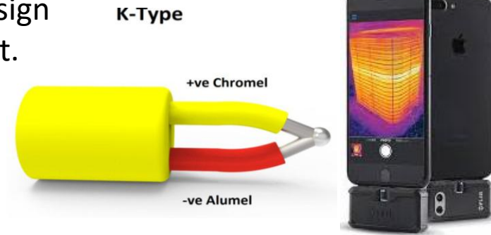
K-type thermocouple and thermal camera for measuring reactor temperature
