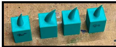
Revised 3D-printed release pins (1/4 scale)
