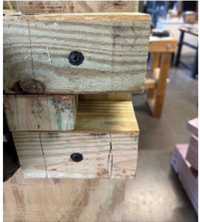
Figure 17: Short feet screwed on the plywood with blocks to hold the wheels.
